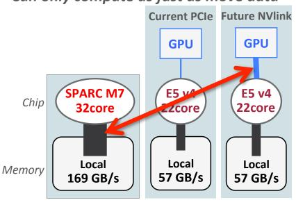
Bandwidth lines to scale GPU compute often stalled by lack of bandwidth
